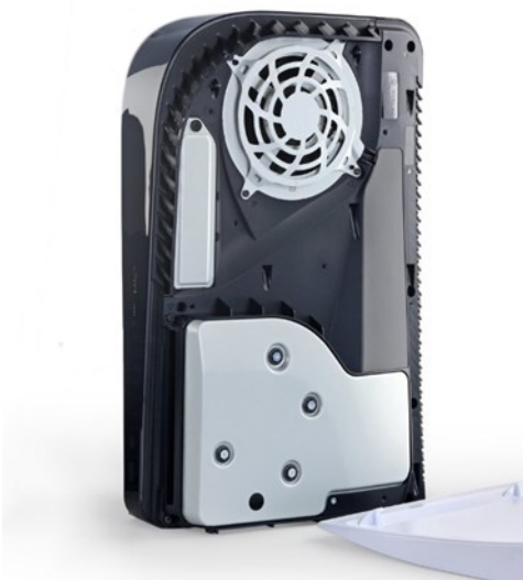
PS5 console with side panel removed
